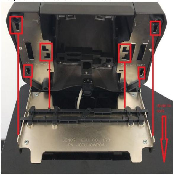
4. Once in position you will need to slide the unit forwards/backwards to be able to lock it in position.
