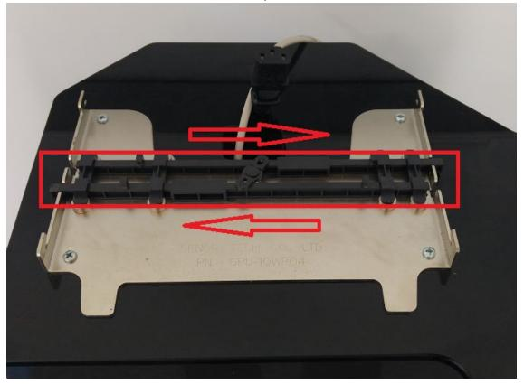
2. Place the unit on the kiosk connecting power and ethernet cables.
